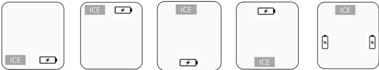
Figure 6.2: Options for the positioning of ICE and battery
